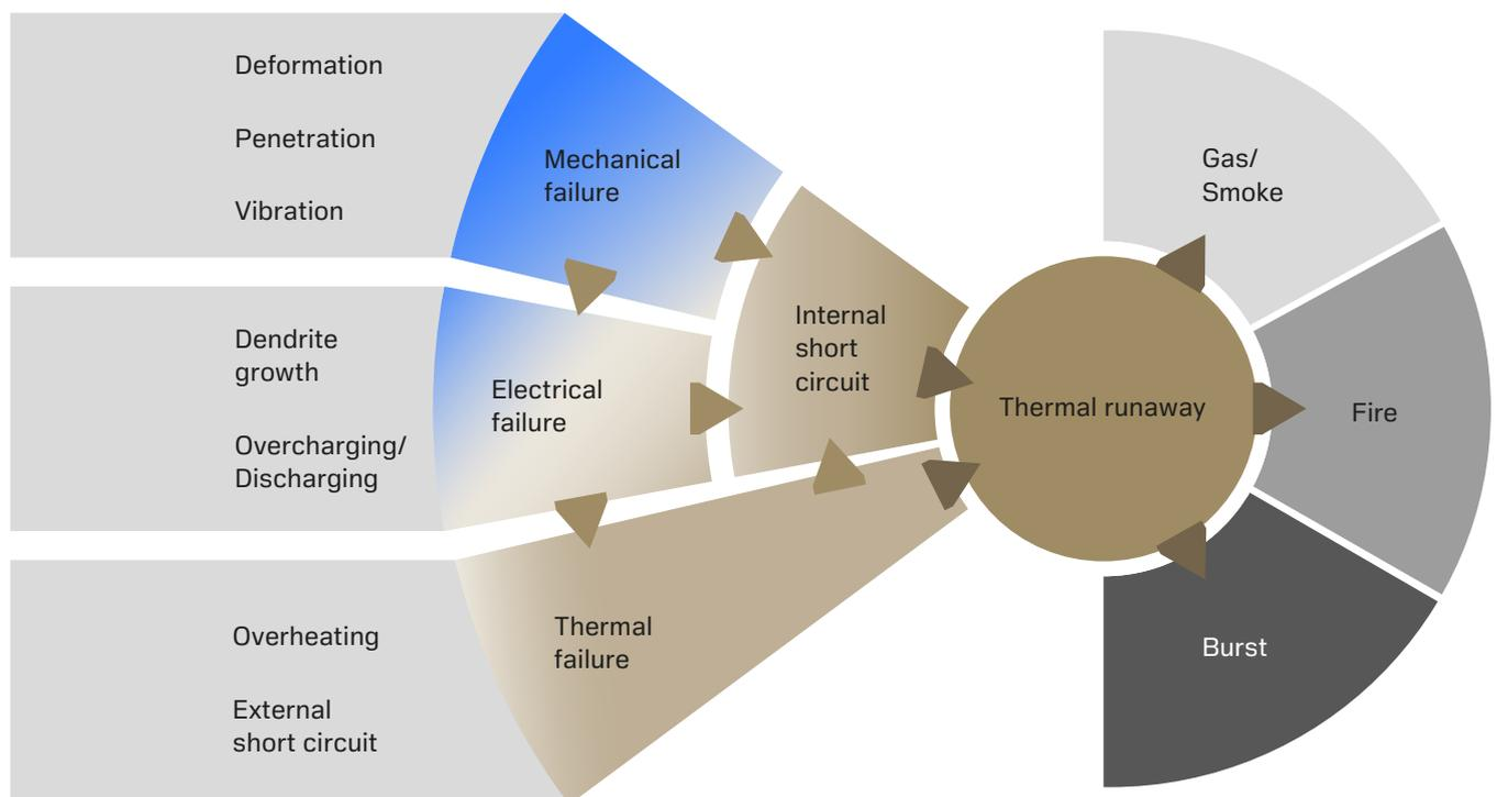
It should be noted that lithium-ion batteries are available in different sub-chemistries, which are not all equally susceptible to thermal runaway. Different sub-chemistries include LFP (Lithium Iron Phosphate), NMC (Nickel-Manganese-Cobalt), NCA (Nickel-Cobalt-Aluminum Oxide), LCO (Lithium Cobalt Oxide). Heat release rates, ignition temperatures, and gaseous release type varies from chemistry to chemistry.
