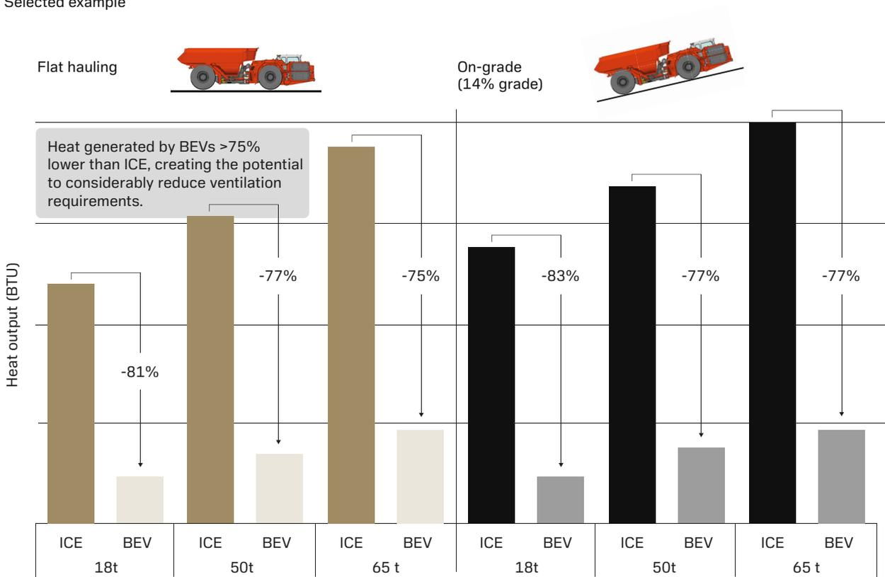
Note: This chart does not account for regenerative braking, which may improve thermal efficiencies by 5–15% depending on cycle parameters.
