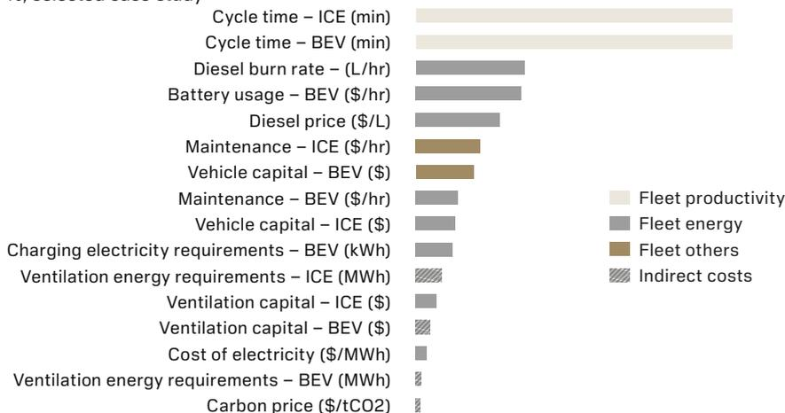
In addition to battery costs and average battery power, the other major key lever in the business case for BEVs is fleet productivity. BEVs benefit from faster acceleration and speed on upramp profiles.
