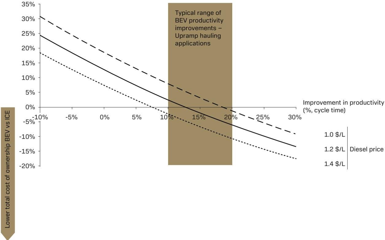
As an example, Figure 18 shows an output of Sandvik simulation tool. This model examines haulage profiles (grades/distances) and mine data inputs such as shift duration, production targets, and size of equipment to estimate energy and battery service requirements through physics-based calculations, and also provide optimized (and configurable) battery charging and swapping schedules.
