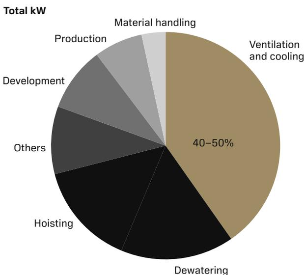
Typical sources of underground mine heat generation
