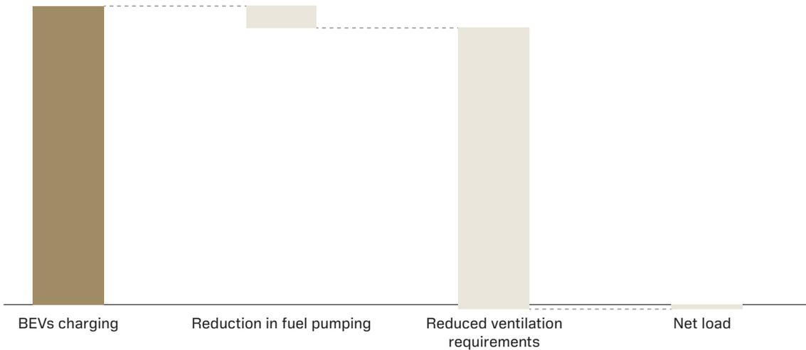
**When optimized, we have found that the introduction of BEVs may be power-neutral given the reduction in ventilation and cooling power requirements.**
