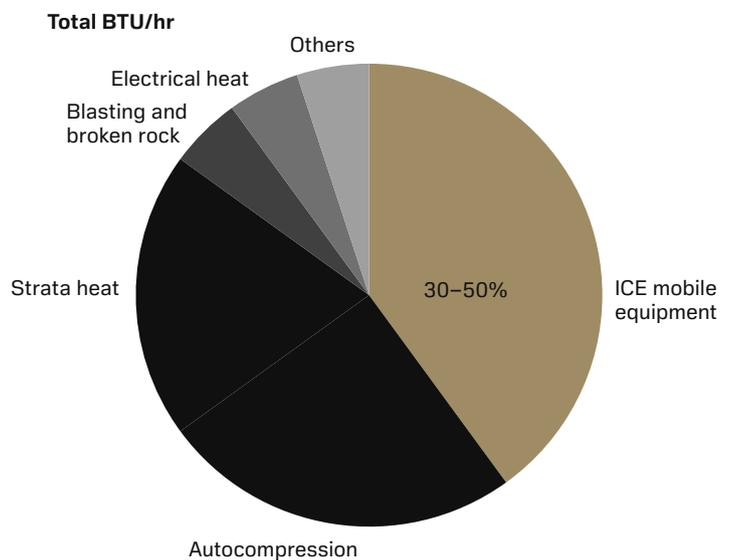
One driver for the reduction in ventilation requirements is the reduction in heat generated: that BEVs use energy stored in the batteries at 80%–90% efficiency when performing work, whereas with ICE equipment, only 20–30% of the fuel energy (diesel) is converted to actual work, the rest being lost to heat. Energy efficiencies and heat losses are further detailed in GMG's 2018 paper "Recommended practices for Battery Electric vehicles in underground mining".
